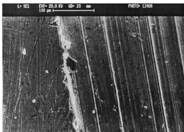
Fig. 16 Micrograph of the disk subjected to diesel as lubricating fluid
